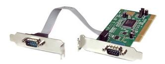
This 2 Port 16550 Serial Card can be installed in a PCI slot to add two serial ports - a cost-effective solution for connecting any new serial device or old legacy serial device, with data transfer rates of up to 115.2 Kbps. The serial card features a low profile bracket, suitable for installation in low profile/small form factor computer cases.
